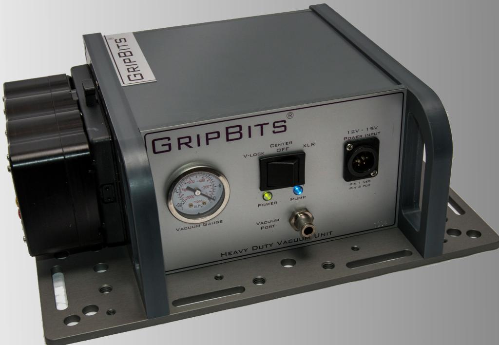
There is a 6mm Hard anodised cheeseplate fitted as standard to the pump to make rigging it a bit easier. All the holes are on 1 inch spacing and some are tapped 3/8x16 and 1/4x20 UNC.
